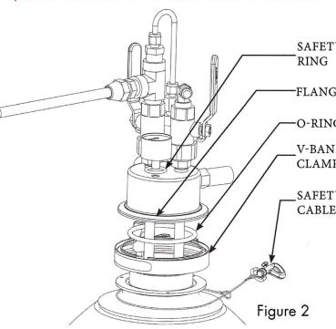
of the hose. If liquid nitrogen is trapped between the valves of the liquid cylinder and the LWD, it has no escape path as it warms and expands. The resulting pressure can cause the hose to rupture and may cause personal injury. The current model LWD is equipped with a pressure relief valve. Previous versions of the LWD must be used with a transfer hose equipped with a pressure relief valve.
